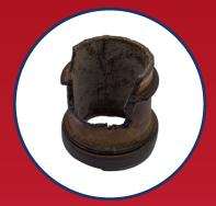
**Eliminate These Failures:** OEM doesent hold on resulting in cracking and deformation.
